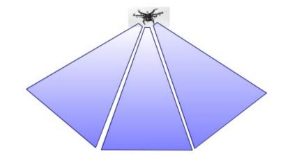
•Glowing/pulsing ball (aka AUGERs oktocopter). Array of diffusers with large opening angles.
