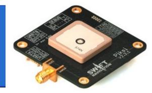
Using GNSS alone: can get to 1.4m accuracy
