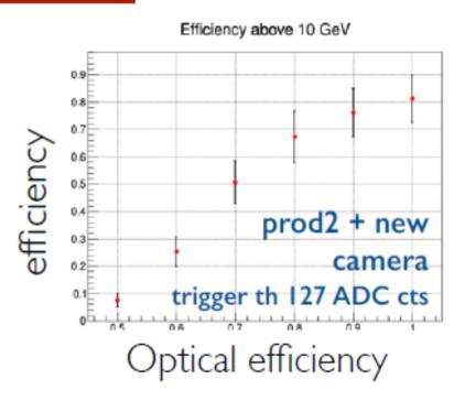
Clear improvement and flat efficiency curve already with trigger threshold 127 ADC counts
