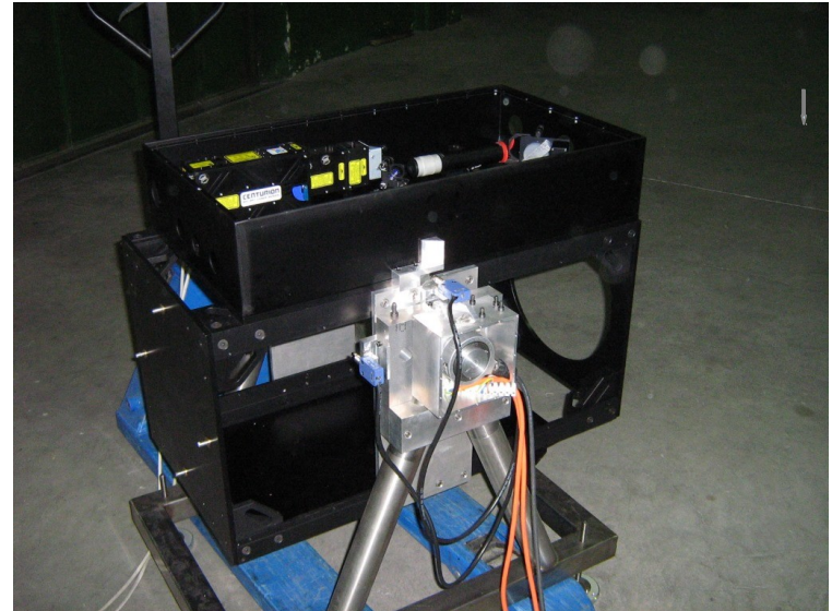
The lidar is mounted on a steering mechanism ...
