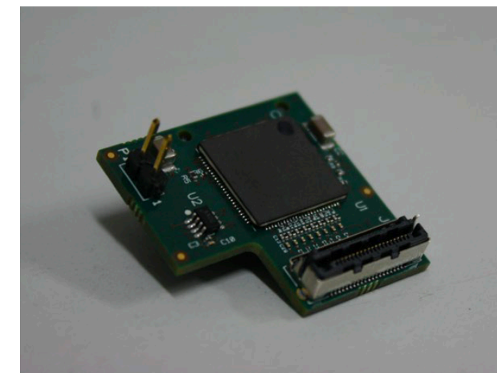
SMART ASIC: Integrated preamplifier attached to SiPM boards
