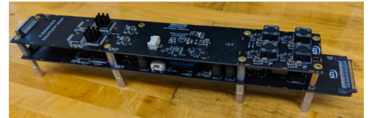
CTC+ CT5TEA FEE module: 16 us storage depth 4 trigger pixels per ASIC Adjustable threshold for each group
