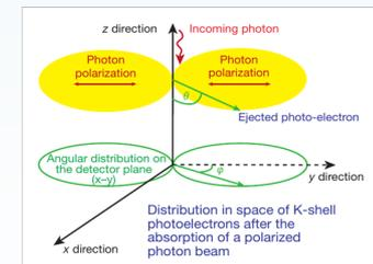
$$\frac{\partial \sigma}{\partial \Omega} = r_0^2 \frac{Z^5}{137^4} \left( \frac{mc^2}{h\nu} \right)^{7/2} \frac{4\sqrt{2}\sin^2(\theta)\cos^2(\varphi)}{(1 - \beta\cos(\theta))^4}$$
