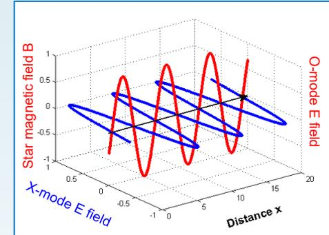
**O-mode**: the E-field oscillates in the k-B plane
