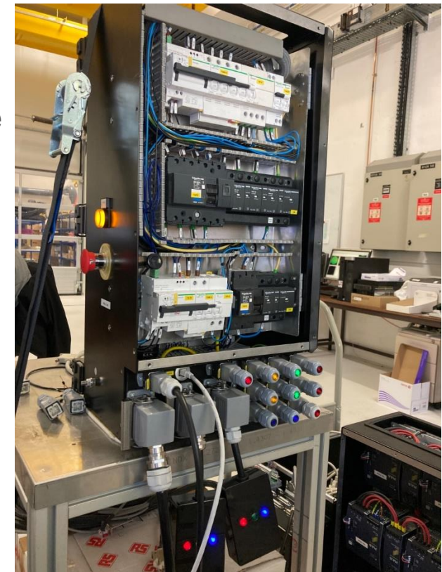
PDB in test with all outputs ON
