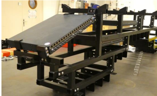
Top mechanical support for Ethernet switches, TIB and UCTS
