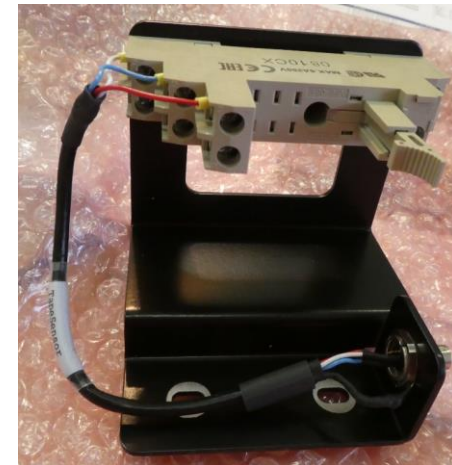
Leak detector with connector located on its mechanical support
