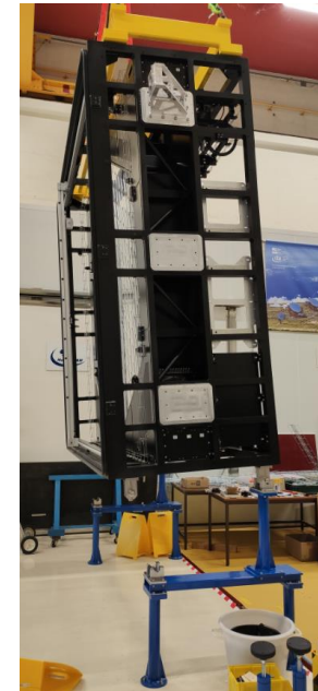
The camera rotates around the axis of the highest legs (blue)
