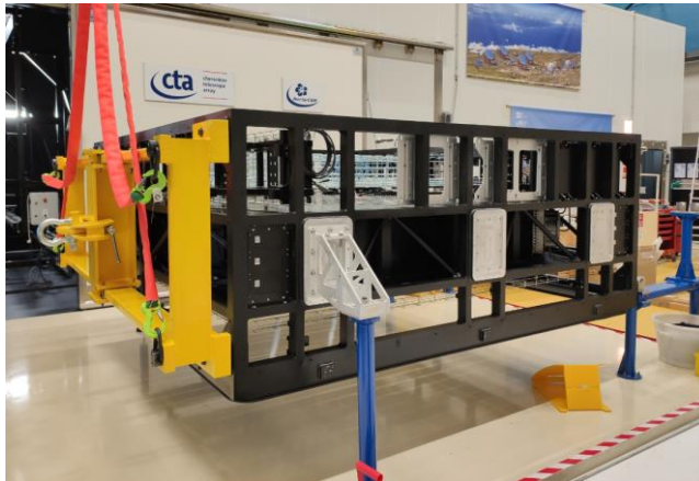
The camera is in horizontal position. The lifting beam (yellow) is at the left
