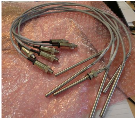
Thermal sensors equipped with their connectors
