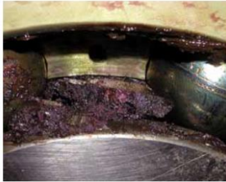
Aged Grease Between Cage and IR
