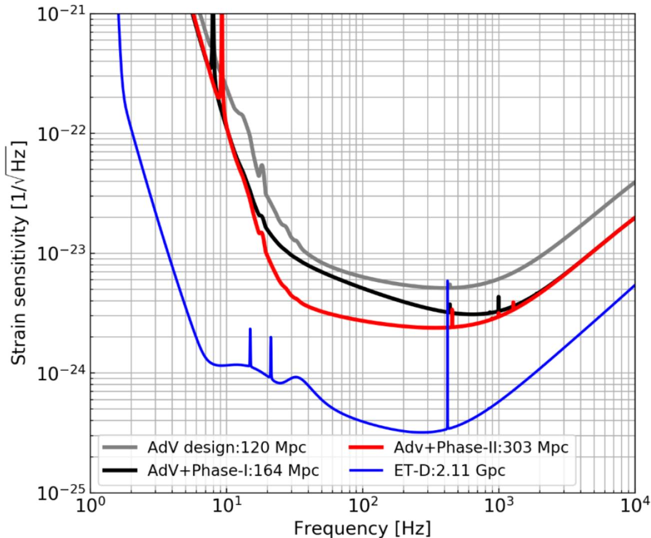
**Figure 3.1:** Expected evolution of the Virgo sensitivity, and BNS range, after the completion of the two proposed upgrade phases. The design sensitivities of AdV and Einstein Telescope are also shown for reference.
