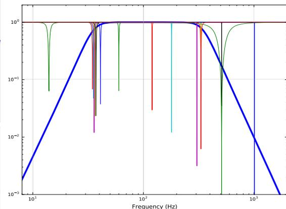
Simple high-low pass filter with notches
