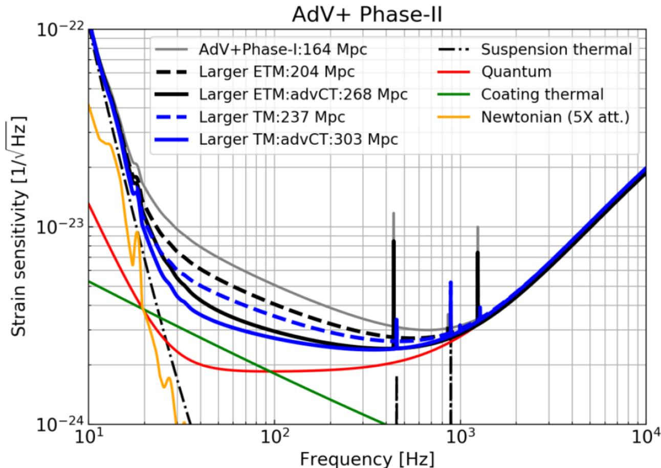
**Figure 3.3:** *Virgo sensitivity after the modification of the arm cavities optical design. The solid curves correspond to a factor of 3 reduction of coating losses with respect to the state-of-the-art (dashed curves). The results for the two possible configurations in which the beam size is increased either on ETMs only, or on all test masses are presented.*
