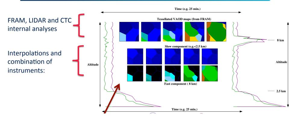
Calculate interpolated extinction cubes (altitude, camera FOV, wavelength, time)
