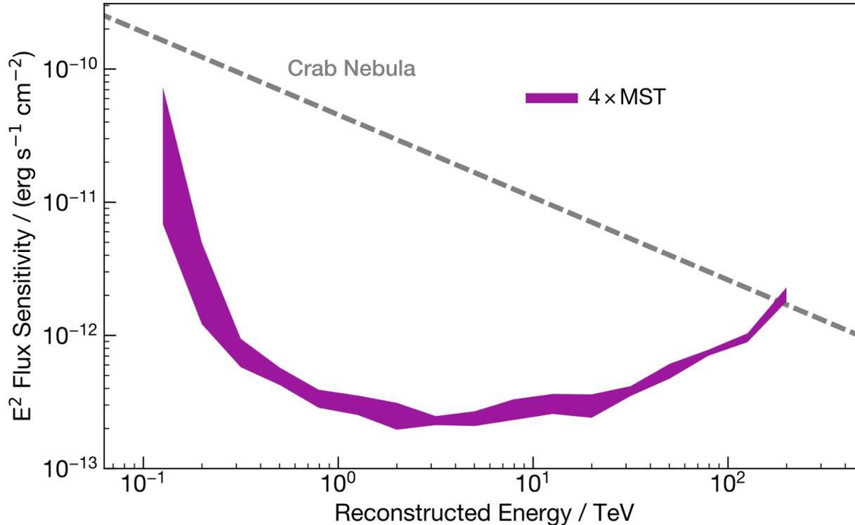
This shows the range of sensitivities spanned by a 4 MST setups at different altitudes (0m & 1000m) and with different baselines (139m & 277m)
