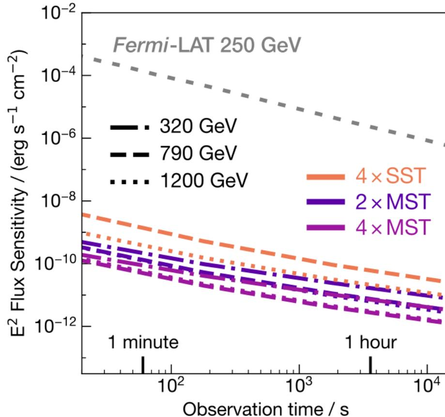
Showing the dimmest source detectable at 5 sigma for a given energy bin as a function of observation time
